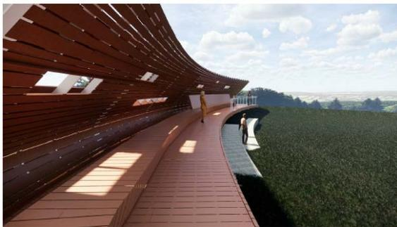
the view of the structure. Structure has no doors and is a west-facing slat wall to provide only nominal shelter from westward wind and direct sun, as it is not intended to be a place of shelter from the elements, but a place to give occupants a chance to be closer to nature: the woodland and the wetlands on the site. The slat wall height is 10’-7” when viewing it from the back (from the west). When viewing it from the lawn that is to the east and at a lower grade, the top of the slat
